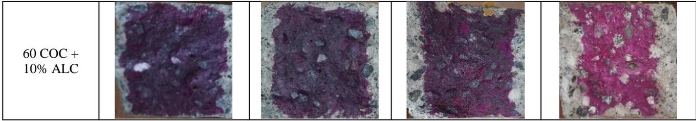
Fig. 3 Accelerated carbonation of various concrete
