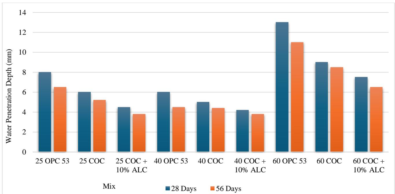
Fig. 1 Water penetration depth of various concrete mix
