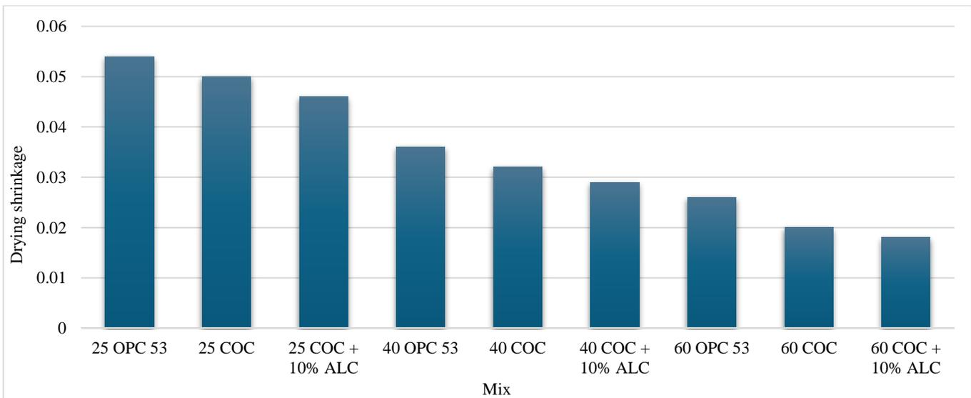
Fig. 2 Drying shrinkage of various concrete
