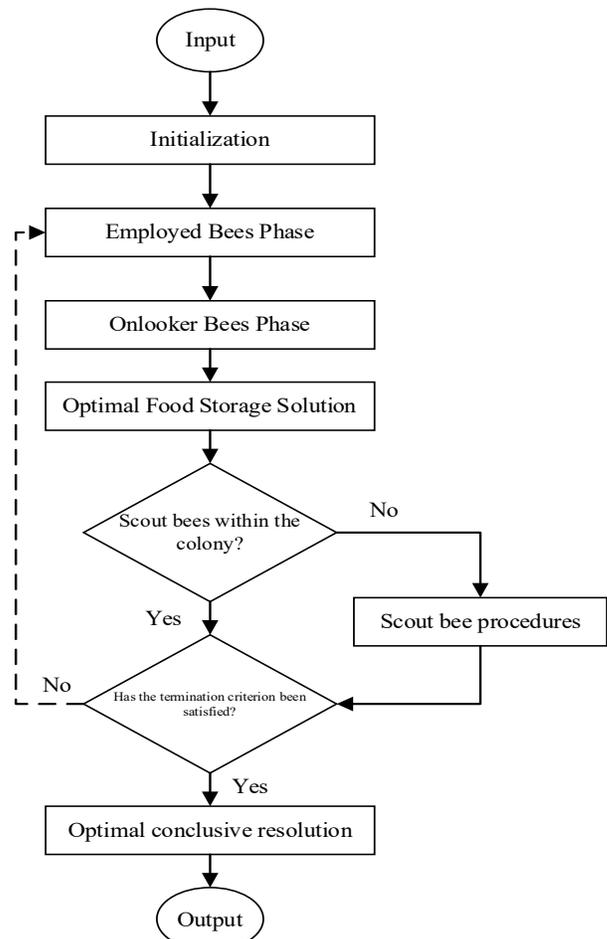
Fig. 3 Bee algorithm standard process, altered from [22]
