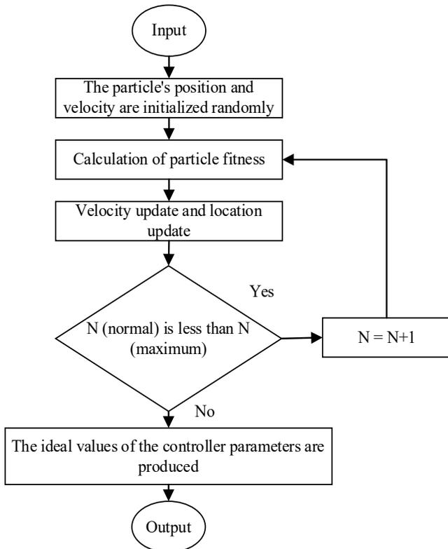
Fig. 2 Particle Swarm Optimization standard process, altered from [15]
