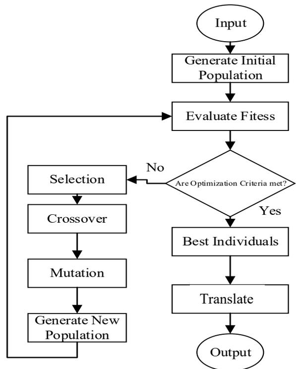
Fig. 1 Genetic algorithm standard process, altered from [12]
